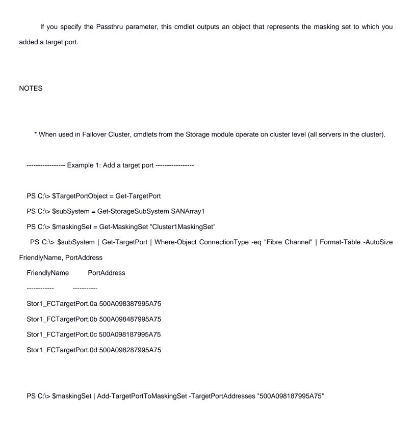
This example demonstrates enumerating the Fibre Channel target ports on a given storage subsystem, and adding one of the target ports to an existing masking set.
